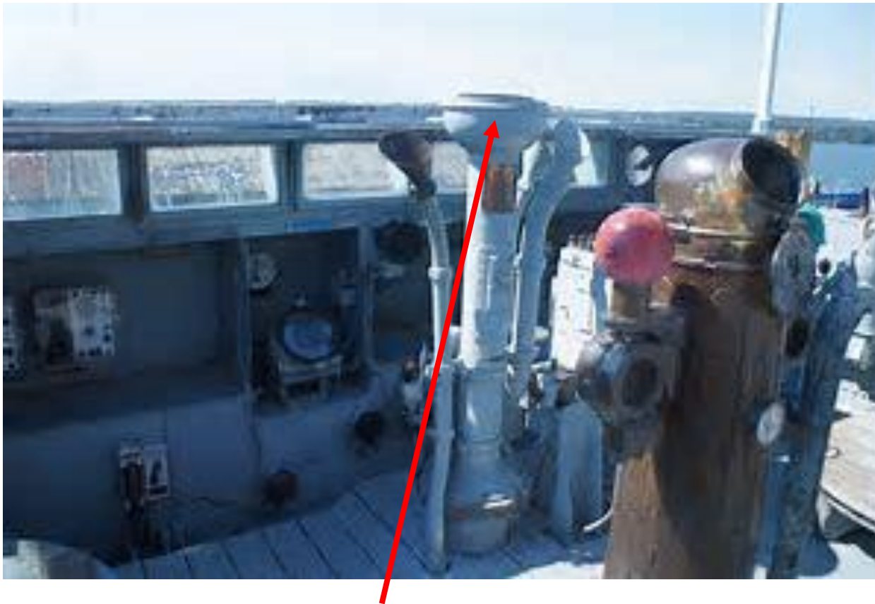
Gyroscopic Compass Repeater It is so tall to see over the forward bridge screen.
